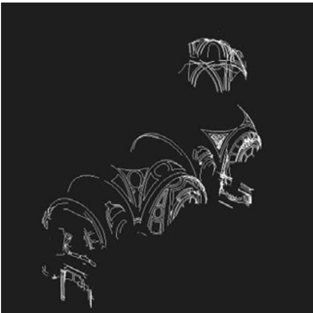
Figure 4. The result of the tridimensional vectorialization of the solid image.
