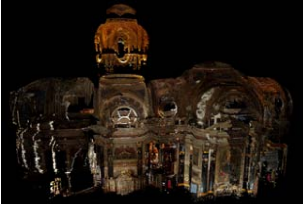
Figure 3. View of the tridimensional cloud of points obtained joining four different laser scanning.
